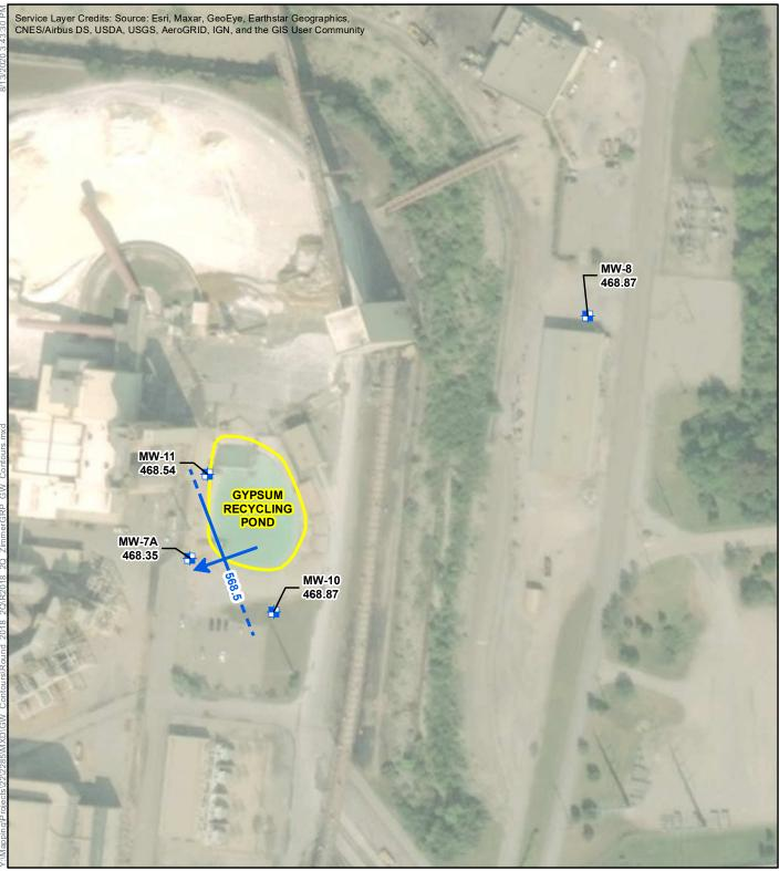
CCR MONITORING WELL LOCATION GROUNDWATER ELEVATION CONTOUR (0.5-FT CONTOUR INTERVAL, FT MSL) INFERRED GROUNDWATER CONTOUR GROUNDWATER FLOW DIRECTION CCR MONITORED UNIT
